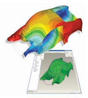
Pro/ENGINEER Mechanica enables validation of the designs and reduces the number of physical prototypes needed.
