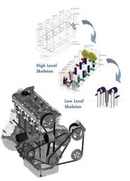
Pro/ENGINEER Advanced Assembly Extension offers capabilities, such as skeleton models, to support top-down design.
